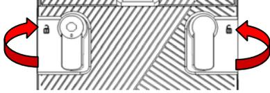
2. To lock the battery by turning down the two knobs. Make sure the battery is securely closed, or you may be unable to turn on the terminal.
