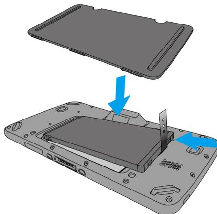
3. Lock the two screws on the battery cover by turning clockwise.
