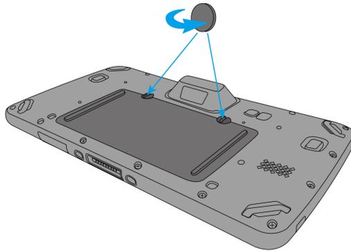
2. Put battery into battery compartment and put back cover.
