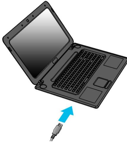
2. Connect the micro USB connector to the micro USB port at the bottom.
