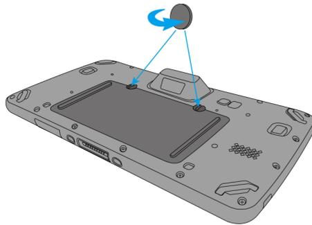
2. Remove the back cover and pull the battery out.
