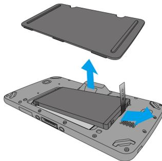
3. Now you can access the micro SD card slot and SIM card slot.
